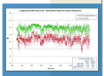
Evaluation of CleanSignal™ in several over the air tests consistently shows at least 3 dB boost in SNR in Wi-Fi applications – effectively increasing the signal range and reception quality.
